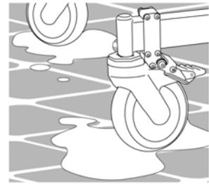
**Transferring onto a Raz AT Shower Chair – ALWAYS** lock all four casters in their outward position (front casters positioned in the forward position/rear casters positioned to the rear) for maximum chair stability. Caster locks **DO NOT and CANNOT** prevent the casters from sliding, and the shower chair from moving, if the floor is slippery. A slippery floor can be caused by dust, water, soap or any substance that does not allow the casters to grip the floor securely.
