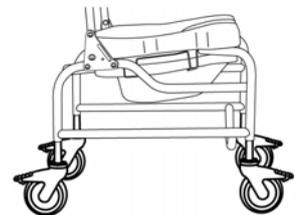
**Transfers should never be attempted with the shower chair positioned on slippery surfaces.** It is recommended that transfers be performed on clean, dry, non-slippery surfaces; a fully-carpeted surface is optimal. Be aware that area rugs and shower mats can slide on floors and thereby present a hazardous surface.
