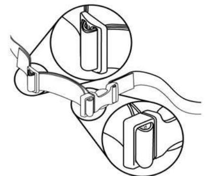
To remove the Adjustable Tension Back Upholstery, release the buckles on the straps.
