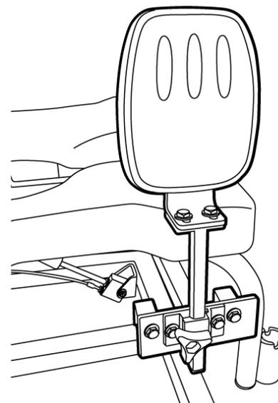
To remove the Leg Adductors, loosen the tri-lobe knob and lift the adductor out of the adductor clamp on the frame.
