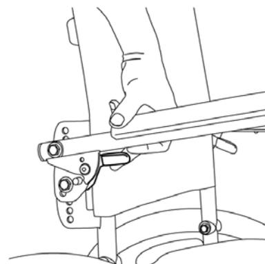
To flip up the locking Armrests, release the arm lock by lifting the blue trigger underneath the armrest tube and lift up the armrest.
